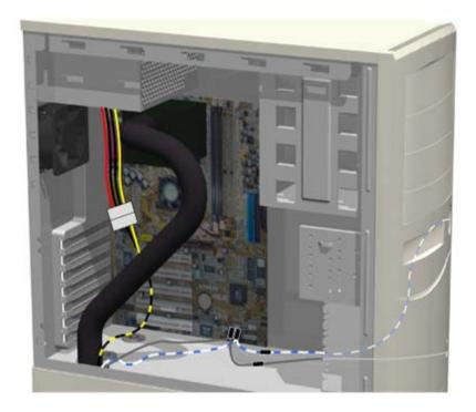
Before you start connecting the wires, you need to make sure that the Thermal bus is positioned so that it does not seat up against the side panel, when you put the side panel back on again. Otherwise the shape of the insulation on the thermal bus will deform, and the insulation capability will be reduced, resulting in possible risk of condensation.
