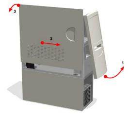
5. Remove the screws for the PC-Casing side covers and slide each side cover towards you and lift up and out, as shown above step 2 and 3.
