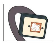
It is of utmost importance that the Microfreezer obtains good contact with the CPU core, a large amount of your subsequent success depends of this.
